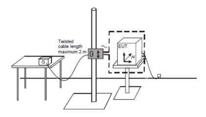
EUT : Equipment under test G : Test Generator
