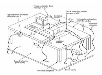
The test setup consists of the test generator, EUT and auxiliary instrumentation necessary to perform DIRECT and INDIRECT application of discharges to the EUT as applicable, in the follow manner:
