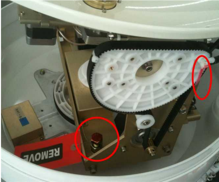
Figure 2-8 Fixed the Screw and Wire Ties
