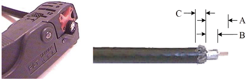
Figure 13 Cutting Technique for Removing Foil in the Braid
