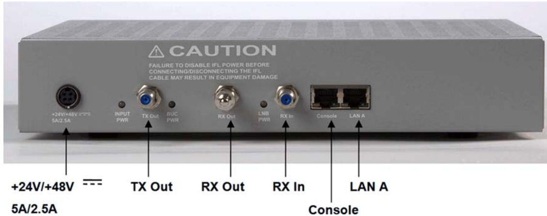
Figure 10 iDirect 3000 series™ Satellite Router Rear Interface Connectors
