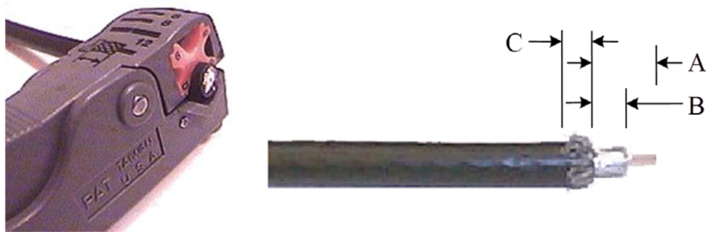
Figure 8. Cutting Technique for Removing Foil in the Braid
