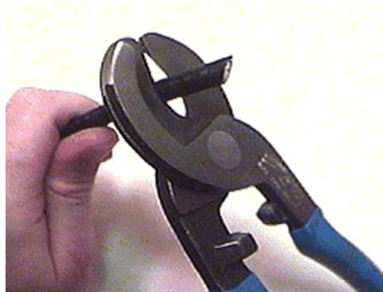
Figure 7. Coax Cable Cutting Technique
