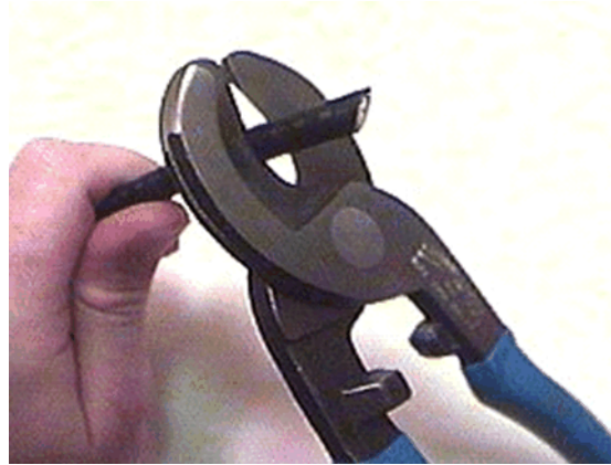
Figure 9 Coax Cable Cutting Technique
