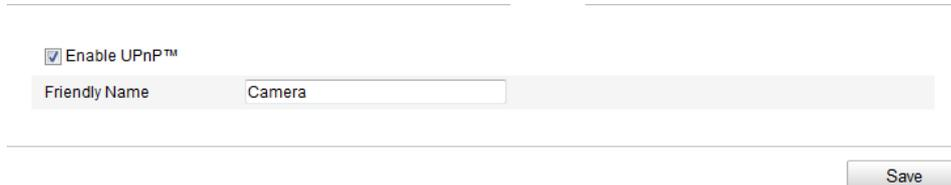
The screenshot shows a web-based configuration interface for UPnP settings. At the top, there is a checkbox labeled "Enable UPnP™" which is checked. Below this, there is a "Friendly Name" label followed by a text input field containing the word "Camera". At the bottom right of the form area, there is a "Save" button.
