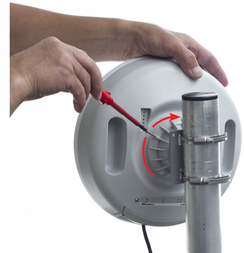
11 While holding the StationBox in desired position, tighten the Nut as much as you can. Optional: To secure the position, use Security Screw that cuts in the Ball part of the bracket.
