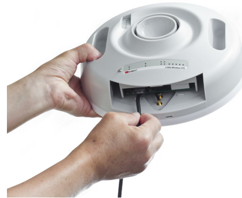
6 Connect the ethernet cable. In case of more cables, knock off the premolded positions in the Cover.
