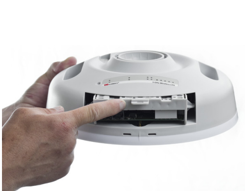
4 Insert the Chassis into the StationBox. Insert pigtails first, then slide the Chassis.
