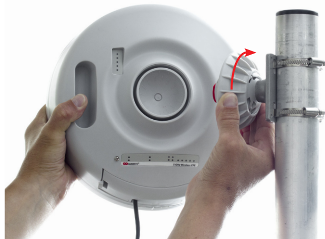
9 Attach the StationBox to the Bracket and slightly tighten the Nut. You should be able to move the StationBox.
