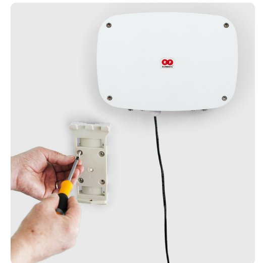
8 Installation on the Wall. Attach bracket to the wall using wall plugs and screws. Then install the enclosure and secure the M4 screw.
