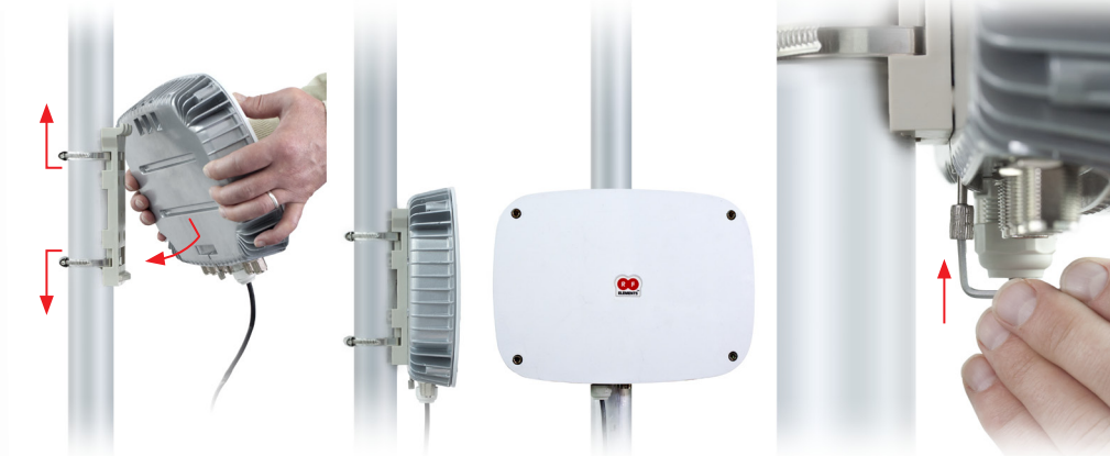
6 Attach bracket to the mast using hose clamps. Clamps shall be as much to the outer edge of bracket, as possible.
