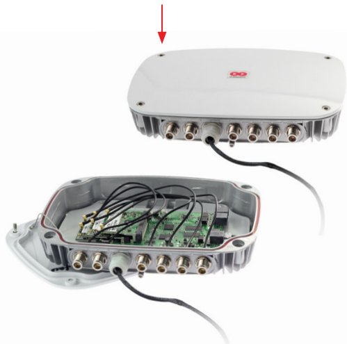
5 Close the enclosure and tighten the screws.
