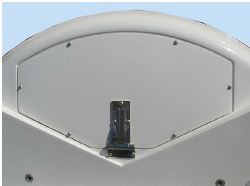
Figure 2-8: Radome Base Service Hatch
