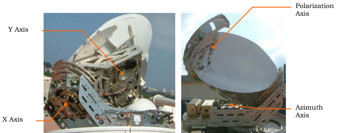
Figure 2-9: Pedestal Axes
