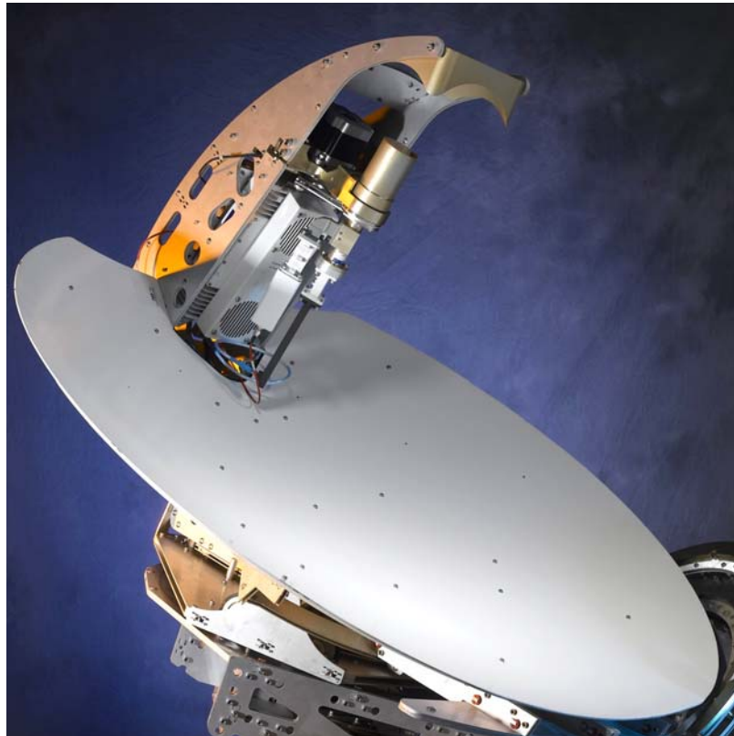
Figure 2-16: Antenna Reflector and RF Front-End
