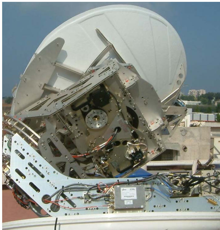
Figure 2-4: Above Deck Equipment (ADE) – sheet 3 of 3
